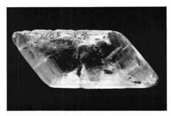
FIGURE 4. Detail of a recently collected Mepal selenite crystal showing growth (or dissolution) steps on {010} and striations on {111}. Crystal is 5 cm in length.
